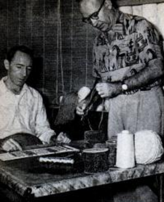
Experimenting with yarns and woods, the two men develop an original pattern which is then set up on loom. Felver uses design card as he selects each strand, which is drawn through loom by Wisroth using a special tool
